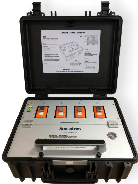
Docking-Station Adjust and Calibration station
